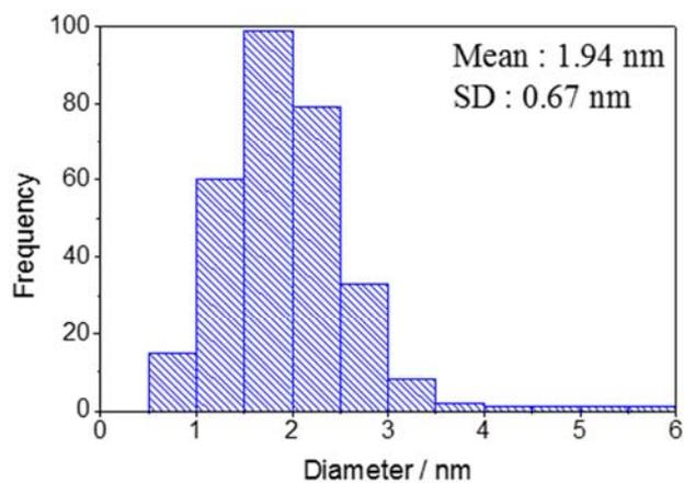
Schema d: TEM<sup>¥</sup> of catalyst D (Au NPs/TiO<sub>2</sub> – prepared by impregnation)
