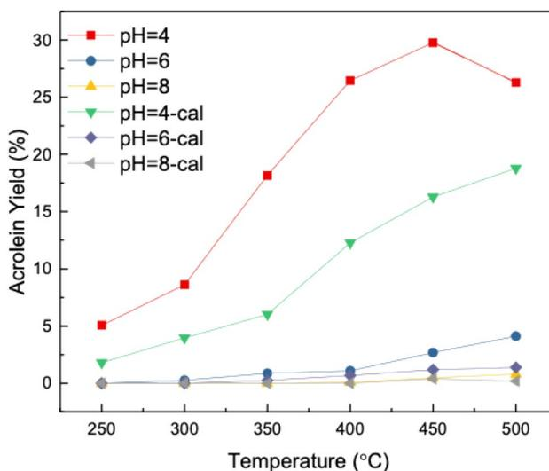
**Fig. 10** Acrolein yield over BiMoOx-4 at different conversions under microwave heating and conventional heating (0.2 g of catalyst, propene:oxyg en:nitrogen = 1:2:97, flow rate = 50 mL min<sup>-1</sup>)
