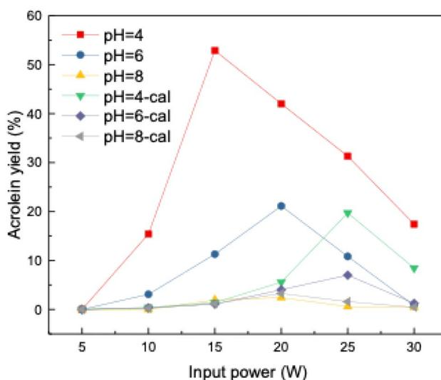
**Fig. 9** Acrolein yield under conventional heating (0.2 g of catalyst, propene:oxyg en:nitrogen = 1:2:97, flow rate = 50 mL min<sup>-1</sup>)
